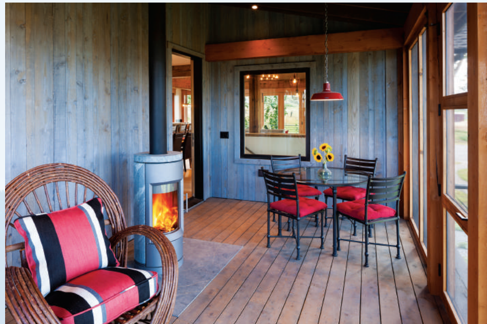
Located off of the great room, a covered porch helps keep the mosquitos at bay even while allowing fresh air to circulate. The fireplace is made from soapstone, and rotates on an axis to more evenly distribute its heat.
